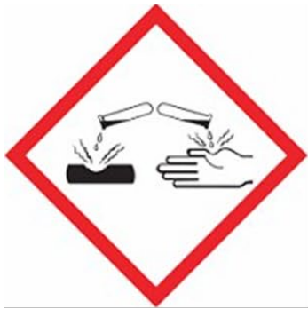
Skin Corrosion Eye Damage Corrosive to Metals
